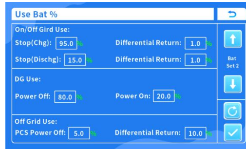
Figure 8 Battery SOC configuration
