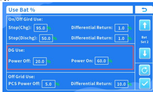
Figure 16 Generator SOC start/stop configuration
