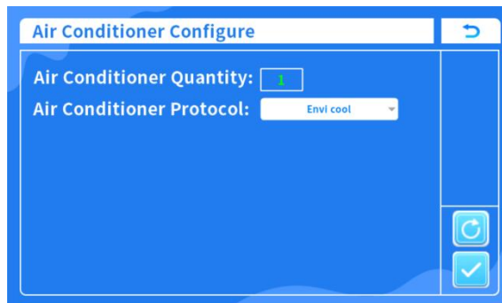
Figure 25 Air conditioning configuration
